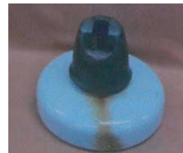
Rust appears on cap due to surface current
